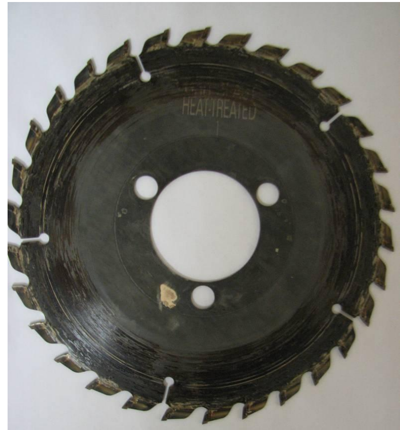
Coated / Gritblasted / Heat Treated @ 8400 lineal feet
