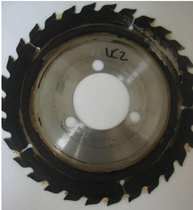
Uncoated @ 7000 lineal feet (time of failure)
